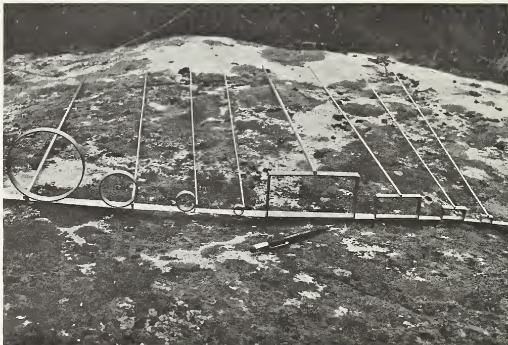
Figure 2.—Set of eight frames used in microplot study. The largest rectangle is 2 by 4 inches.
