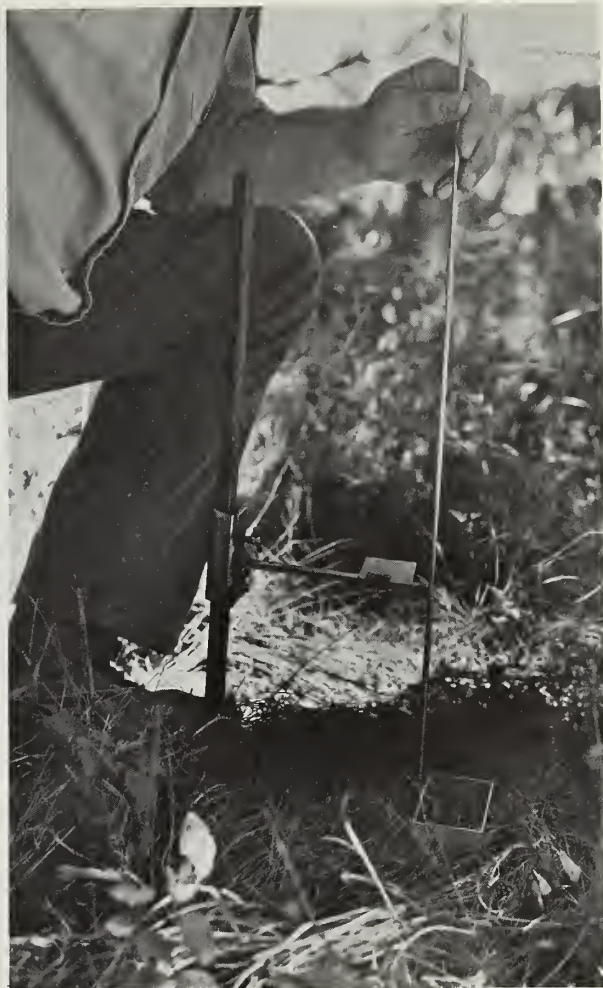
Figure 3.—Sliding metal arm used to position microplot frames in the same place.
