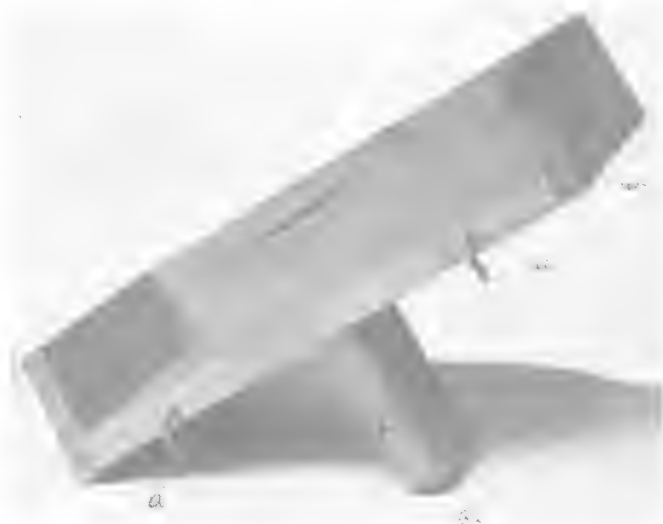
Fig. 20. Paper "Hod," for Use on Top Edge of Box. a Hooks which engage the top edge of the box. b Cleat beveled at the same angle as the box so that when it is in place the hod is in a horizontal position.
