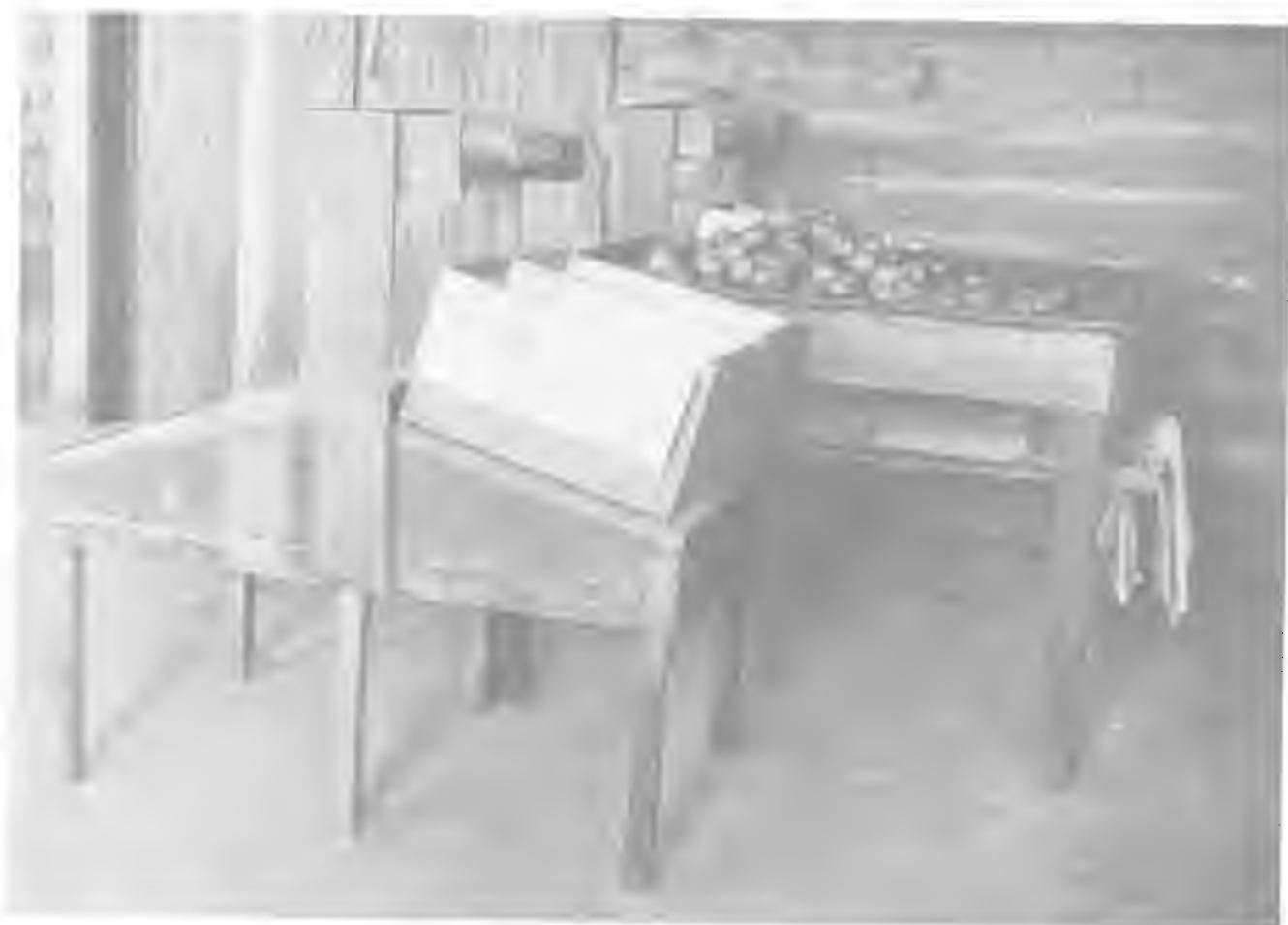
Fig. 18. Table and Bench in Use by Mr. J. H. Estes, Zillah, Wash. Note the shelf for wrapping paper above the boxes, the shelf for cardboard and extra wrapping paper underneath the burlap table, the rack for lining paper attached to this table, and the front incline to the packing bench, to which the packer can shift his packed box to await the attendant. The arrangement shown is for one right handed and one left handed packer.
