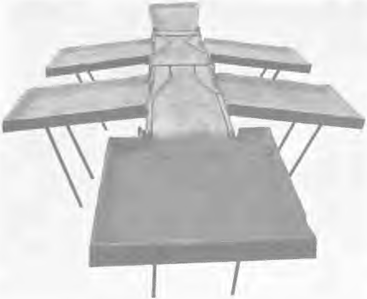
Fig. 13. Gilbert Sorting Belt Receiving Trays in Place.
