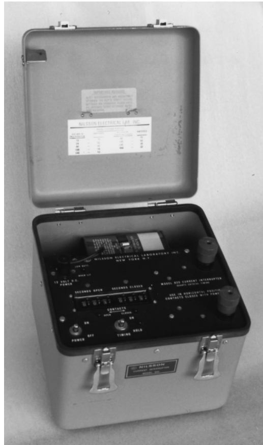
Figure 6.10 Quartz crystal controlled current interrupter. (Photo courtesy of Nilsson Electrical Laboratory Inc.)
