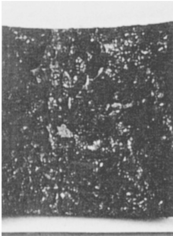
Figure 14.4 Black manganese dioxide deposits on carbon steel caused by metal-depositing bacteria.
