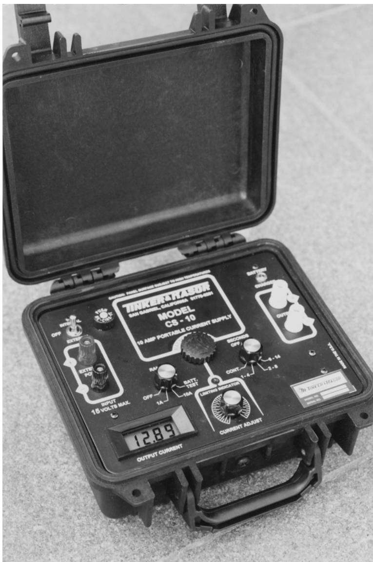
Figure 6.18 Portable battery operated D.C. power supply. (Photo courtesy of Tinker and Rason.)
