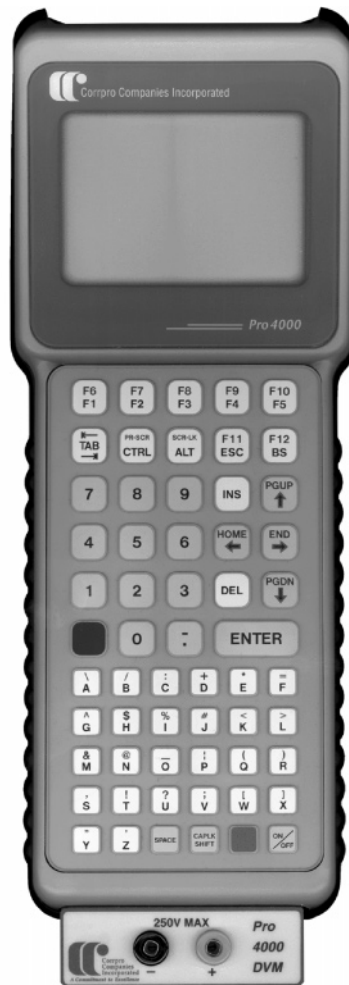
Figure 6.6 Electronic data recorder. (Photo courtesy of Corrpro Companies, Inc.)
