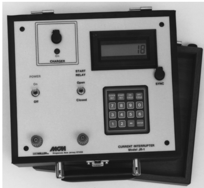
Figure 6.11 Programmable current interrupter. (Photo courtesy of M. C. Miller Co.)
