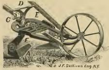
Note. -A. The cast-steel Knife, corrugated so as to be set at any angle required. C. Thumbscrew to raise or lower the handle. D. Ridged brace for supporting and regulating the handles E. Thumb-screw for regulating blade shanks.
