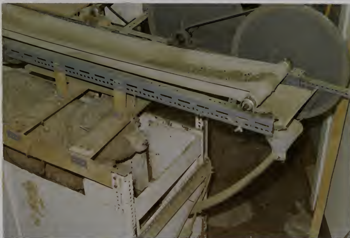
Figure 1a. Continual Feeder Showing Delivery Belt, Delivery Funnel and Tube, and Pulley Drive System
