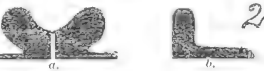
Rear sight on barrel; blued; showing platinum line in center; with notch; (a) front view; (b) side view; extreme height, 9/32 in.; extreme breadth, 9/32 in. The object of this sight is to enable one to more readily find the center of the globe.
