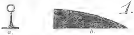
Front sight, bead shape; blued; pin of platinum driven in bead; (a) front view; (b) side view; 7/32 in. in height.
