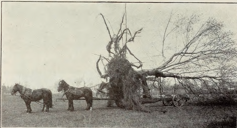
Ready for the Road. —The tree is loaded with shortest branches and roots on top, so it can go under electric wires, which are lifted by a T-pole. Four to eight horses or traction engine, broad tires, and planks over lawns, enable heavy trees to be moved. Rope and tackle or windlass are also used in difficult places.
