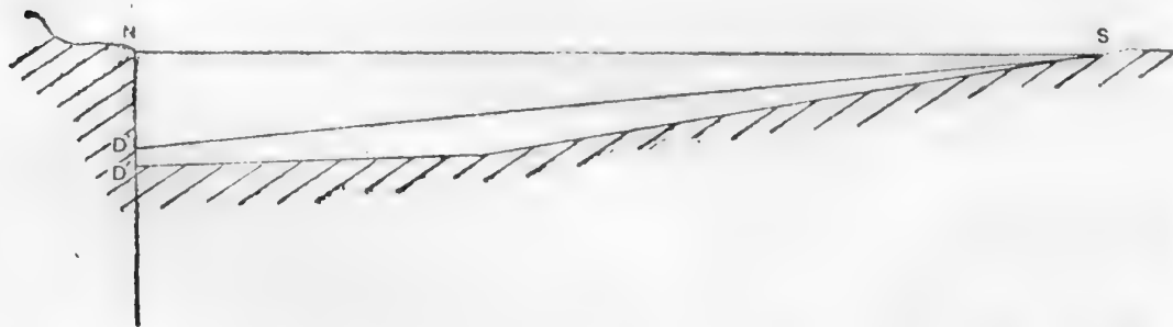
FIG. 5.—Showing the effect of separate compensation of the trough on the interpretation of the deflections. If NDS represents the cross section which would be indicated if there were no separate compensation, then ND'S represents the interpretation if compensation is considered.
