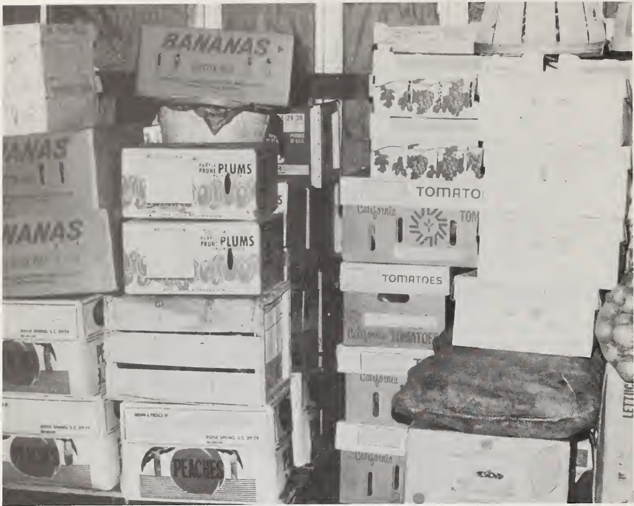
Figure 1.--Typical array of shipping containers for delivery to retail store. Incompatibility in sizes and shapes leads to difficulties in stacking.
