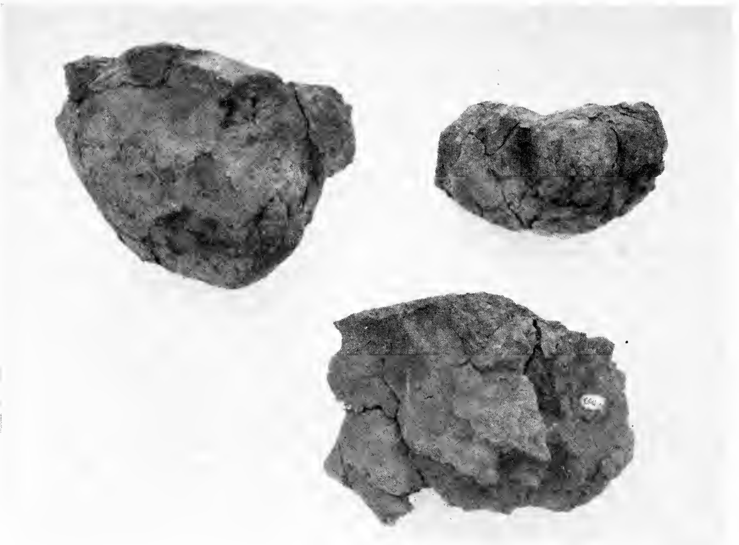
Fig. 2.—Side elevations of three major fragments showing weathering effects. The upper surfaces of all are original dimpled surfaces. Top left: spheroidal core after loss of up to 2 in. by exfoliation from the underside. Bottom right: upward wedging cracks sub-divide the mass into individuals which weather spheroidally. Top right: cracking and weathering advanced, a well-defined spheroid in the middle. The two large specimens are one foot wide.
