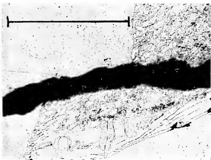
Figure 3.—Photomicrograph showing faulting of a kamacite/plessite interface in Yarri meteorite. Scale bar 1 mm.
