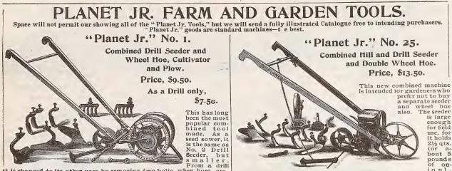
From a drill it is changed to its other uses by removing two bolts, when hoes, etc., can be quickly attached. It is an excellent seed sower, a first-class double or single wheel hoe, an excellent furrower, an admirable wheel cultivator, and a rapid and efficient garden plow. It is a practical, every-day, time and labor saver, and a grand remedy for backache. A pair of 6 tooth rakes supplied when specially ordered. **Price, 50e**.
