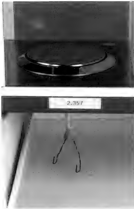
FIG. 3. Underwater weight measurement. Detail of an explant placed in the hanger under the balance.
