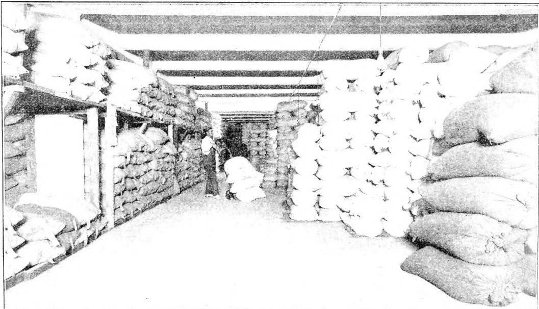
A corner of the second floor, showing method of piling bags of seed. The bags are placed so as to allow a free current of air through them, and all are placed on frames or mats on the floor.
