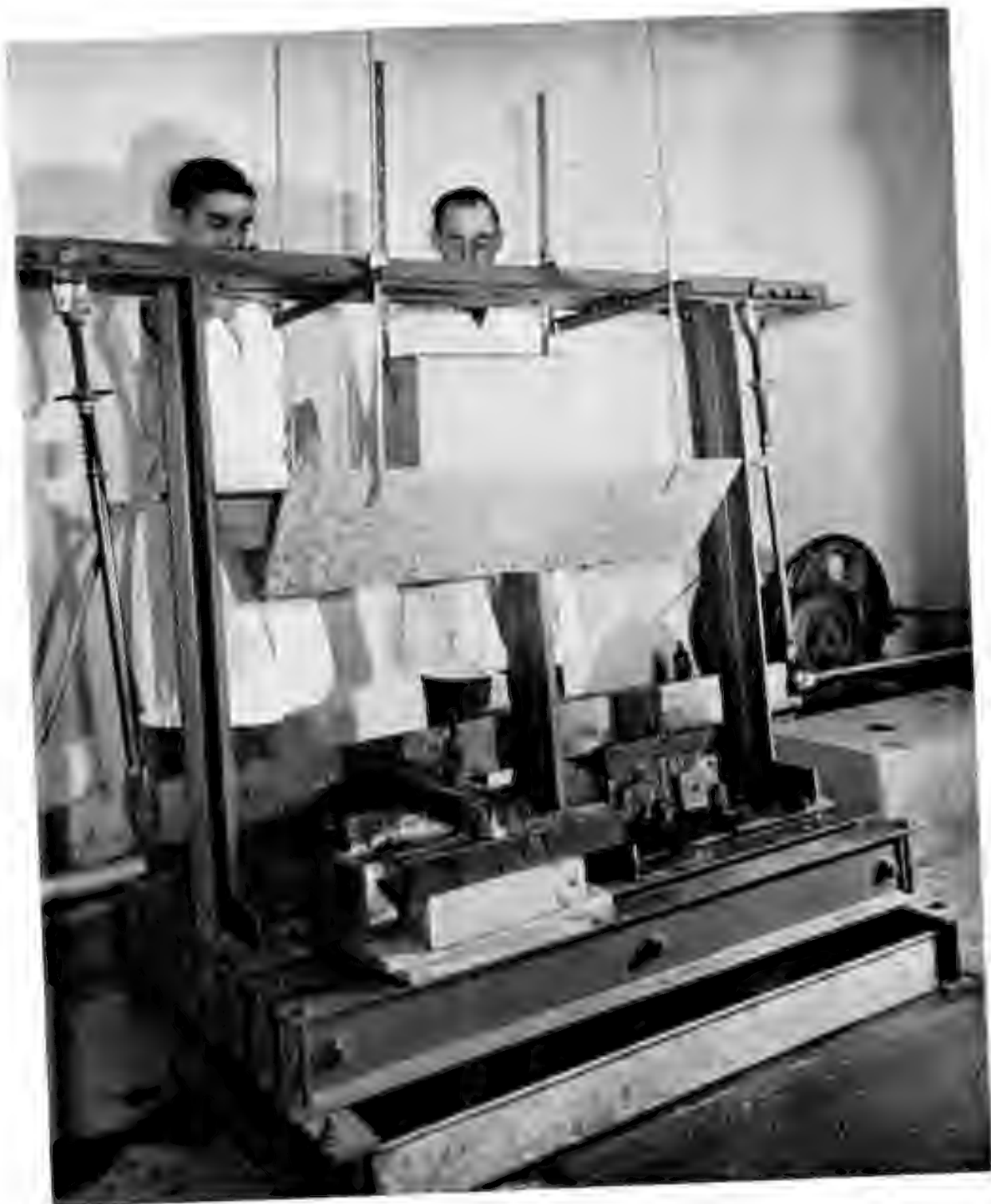
Apparatus for cutting meteorites in South Australian Museum, 1954
