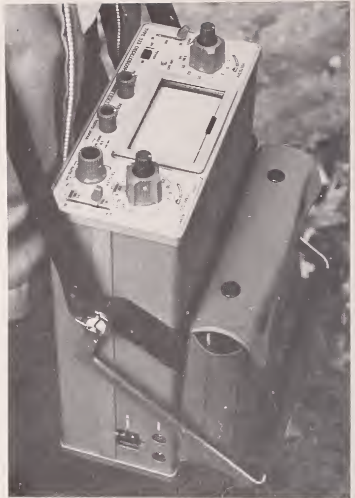
Figure 15. Vertical "flashes" on the oscilloscope screen indicate presence of signal from subject animals. The flash rate identifies particular animals.
