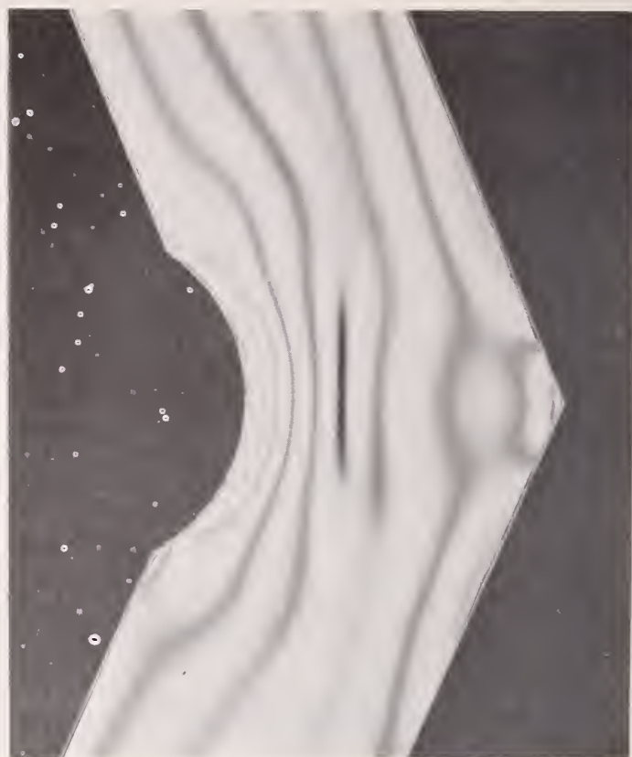
Figure 44. Photoelastic strain pattern around an undercut fillet. Such model work together with photoelastic coating studies of wood corner joints with undercut fillets aided in a study of the effectiveness of undercut fillets in reducing stress concentrations at least at the qualitative level.
