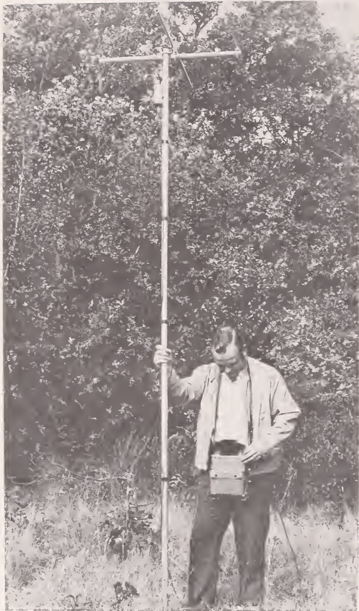
Figure 14. The portable telemetry system includes an antenna, a small receiver mounted under the antenna, and a portable oscilloscope.
