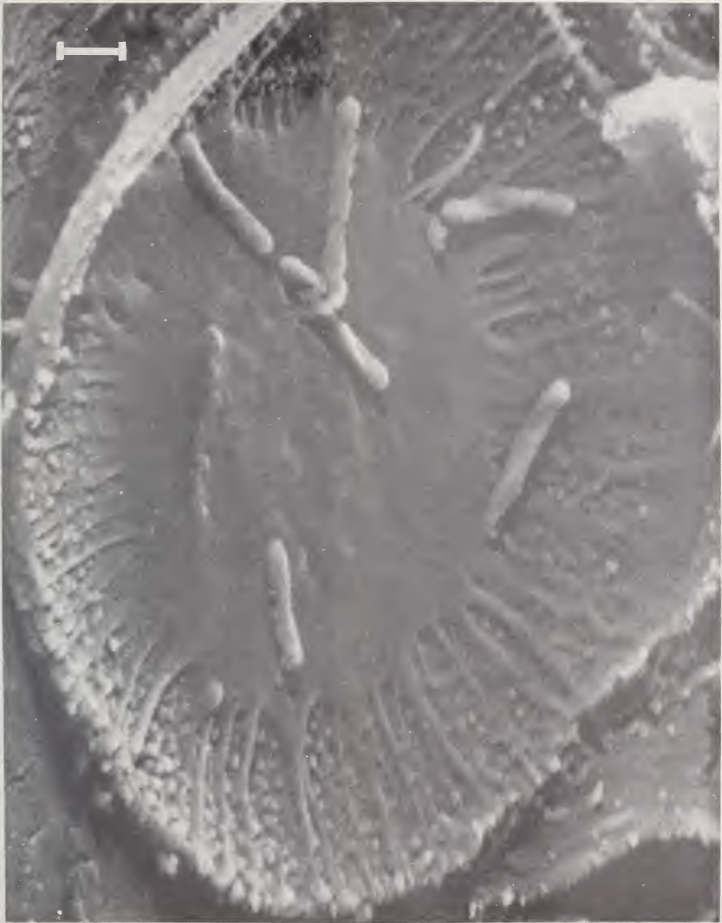
Figure 37. Scanning electron micrograph of surface of pit membrane for wood which had been incubated in a nutrient medium inoculated with the bacterium isolated from white fir wetwood. Bacterial cells are shown on the surface of the membrane which appears intact despite their presence (— = 1 \mu m).
