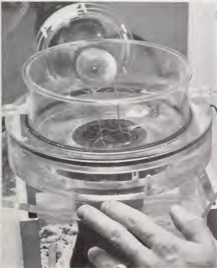
Figure 5. Transpiration of Douglas-fir seedlings is measured to determine effect of seed source and nursery growing conditions on seedling survival under moisture stress.
