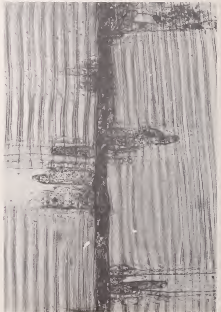
Figure 43. The movement of resin into ray cells results in appreciable absorption by latewood tissue as well as earlywood of southern pine. In both A and B the glue mix was the same.
