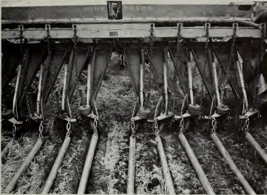
CLOSE-UP OF DRILL SHOWING WEIGHTS AND PIPE DRAGS
