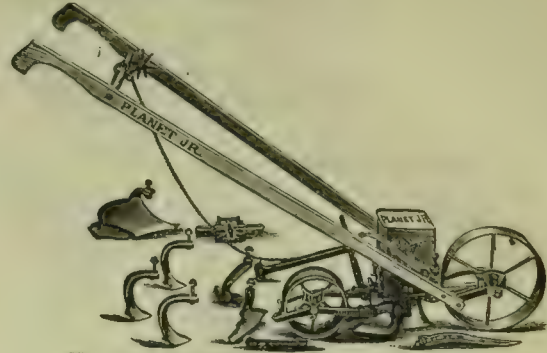
No. 4. Combined seeder and Cultivator.
