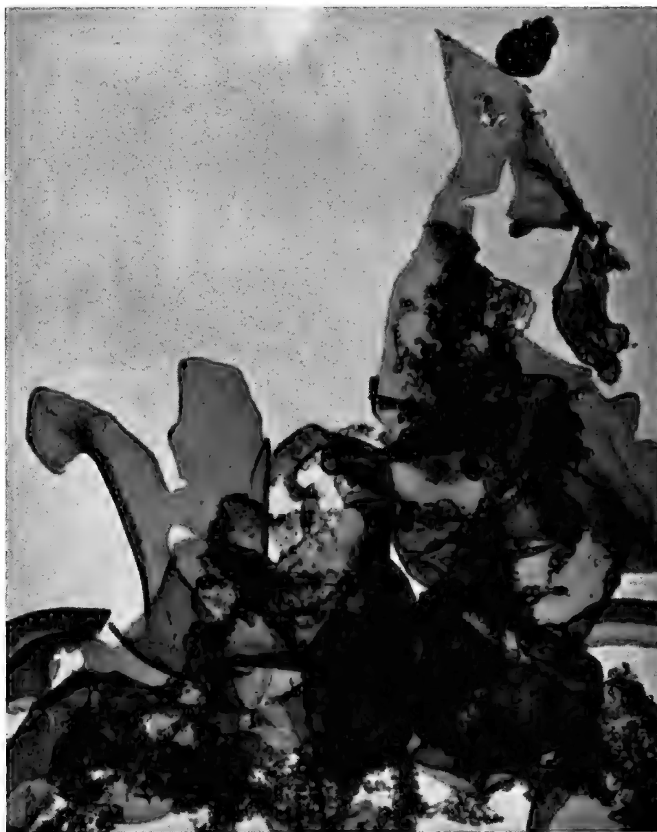
Electron micrograph (12,000 x) of unknown residue after evaporation of the sulphur.
