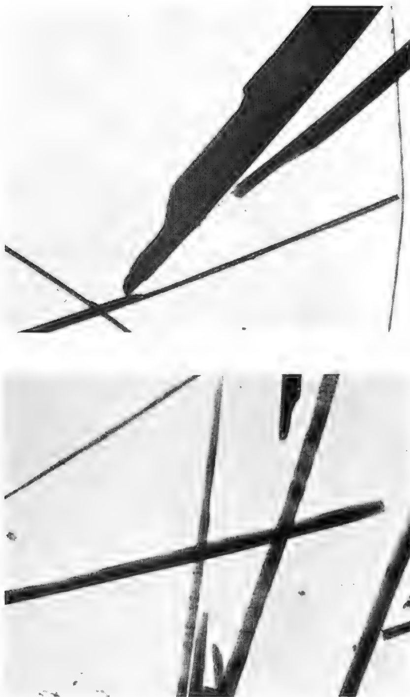
Plate II. Electron micrographs of magnesia crocidolite from Robertstown, South Australia. The top figure (a), at \times 5,000 , illustrates inconsistencies in the fibrous habit and the lower figure, at \times 15,000 , shows the tubular form of the individual crystals.
