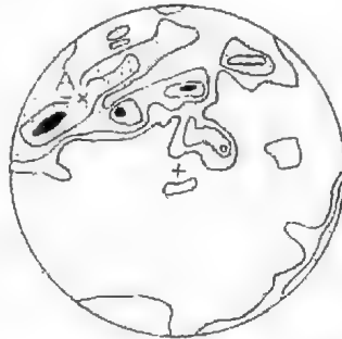
Fig. 3. Quartz orientation diagram of small grains enclosed in a single large grain. The average orientation of the large strained grain is shown as A. Spec. 157-172 220 grains. Contours 1-2-3-4 p.e. per 1 p.e. area.
