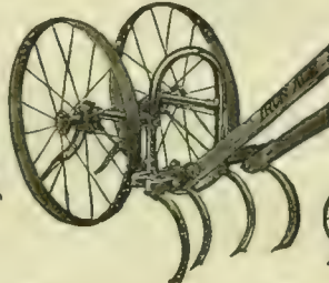
No. 301R. Cultivator teeth can be set to suit the width of rows
