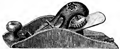
IRON SMOOTH-PLANE FOR DRESSING THE BEVELS TO AN EXACT FIT.
