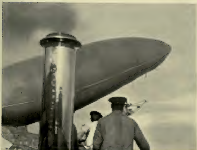
Fig. 5. The after-end of the girder being immersed, the Balloon is in equilibrium in the air, while the guide-rope is being got into the launch.
