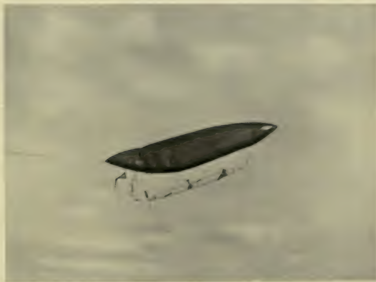
Fig. 4. The Balloon buckling on the escape of gas.
