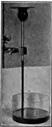
Fig. 103. Apparatus to show respiration of germinat- ing wheat.
