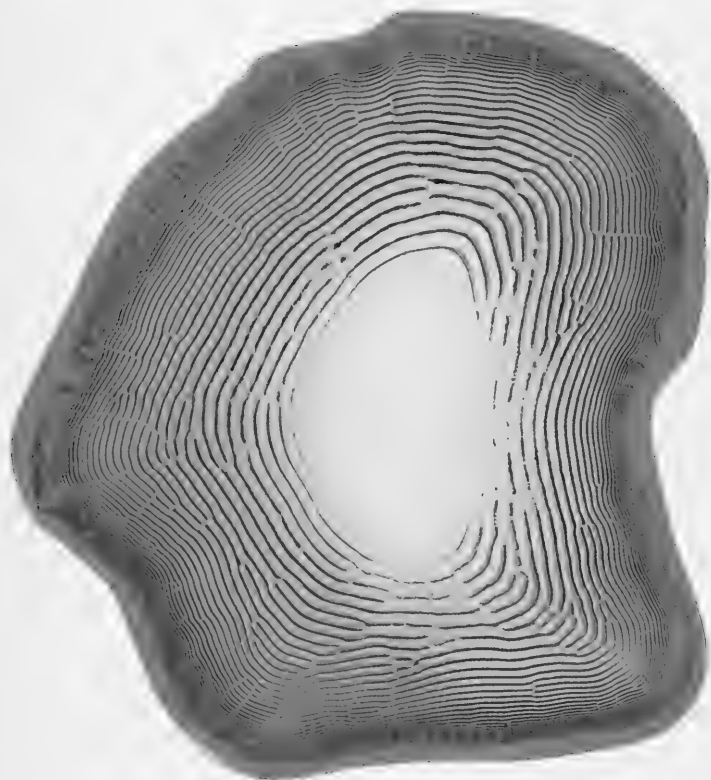
AGATE-LIKE BANDING PRODUCED BY DIFFUSION IN GELATINE. "LIESEGANG'S RINGS"
