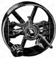
Fig. 238. One form of clutch. The wooden shoes are forced outward against the rim of the wheel, engaging it by friction.
