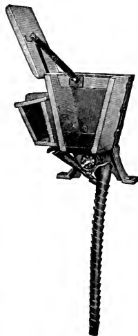
Fig. 141. A section of the seed box of a drill showing location of the grass seed box and a steel ribbon tube.
