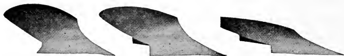
Fig. 108. The three principal types of plows, showing in order the stubble, the general purpose, and the prairie breaker plows.
