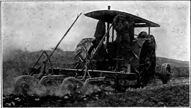
Fig. 236. A small gas tractor plowing. It may be successfully operated by one man.
