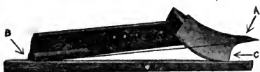
Fig. 111. A share with the proper form at the wing. The contact or "bearing" at C should be about 1\frac{1}{4} inches wide for a 16-inch plow.
