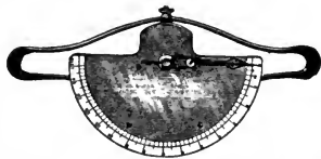
Fig. 198. A direct-reading traction dynamometer.
