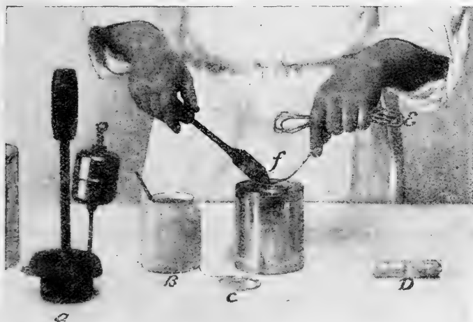
(A) Self-heating capping iron. (B) Flux jar and brush. (C) Solder-hemmed cap. (D) Ammonia bar for cleaning irons. (E) Wire solder. (F) Tipping copper and method of application.
