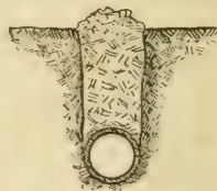
A modern tile drain.
