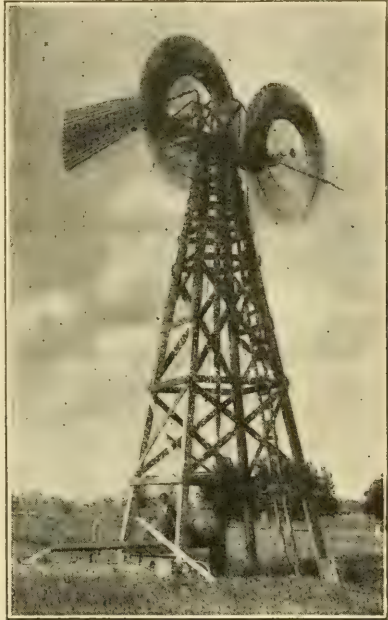
Pumping underground water with a windmill and storing the water in an earth reservoir. This method is adapted to irrigating small areas.
