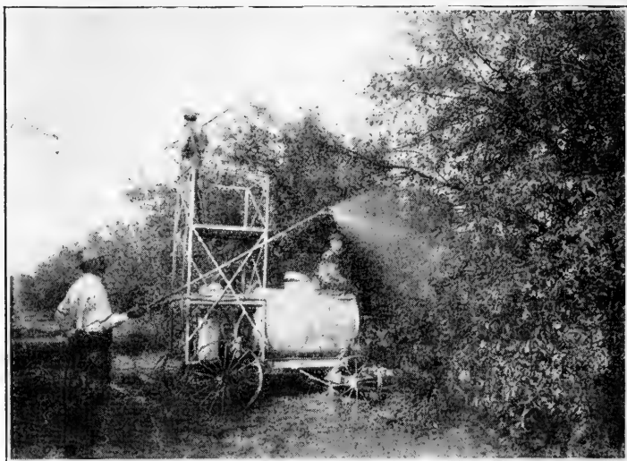
A power sprayer in the orchard. The spray material is forced upon the trees in a fine mist.
