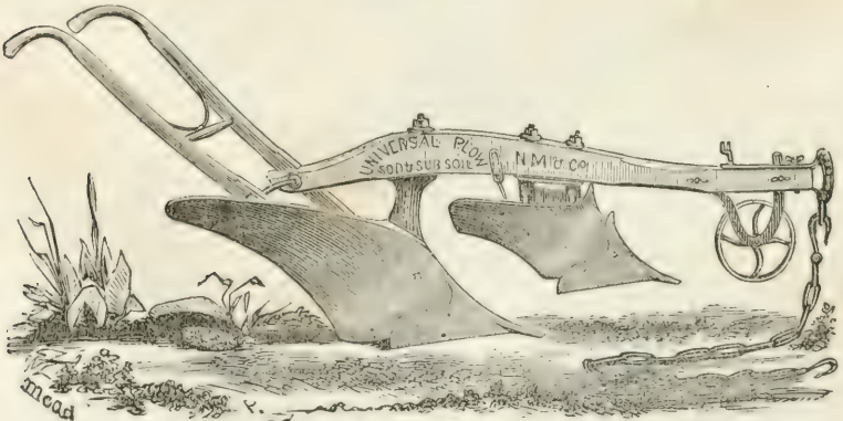
Holbrook's Universal Plow as a "Michigan" or sod and subsoil plow.
