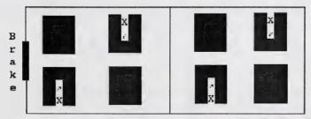
• 2-Compartment, Open Top Type Hopper Cars. Insert probe in the direction of the arrow at an approximately 10-degree angle.
