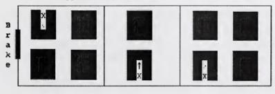
• 2-Compartment, 8-Hatch Type Hopper Cars. Insert probe in the direction of the arrow at an approximately 10-degree angle.
