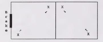
• 4-Compartment, 12-Hatch Type Hopper Cars. Insert probe in the direction of the arrow at an approximately 10-degree angle.
