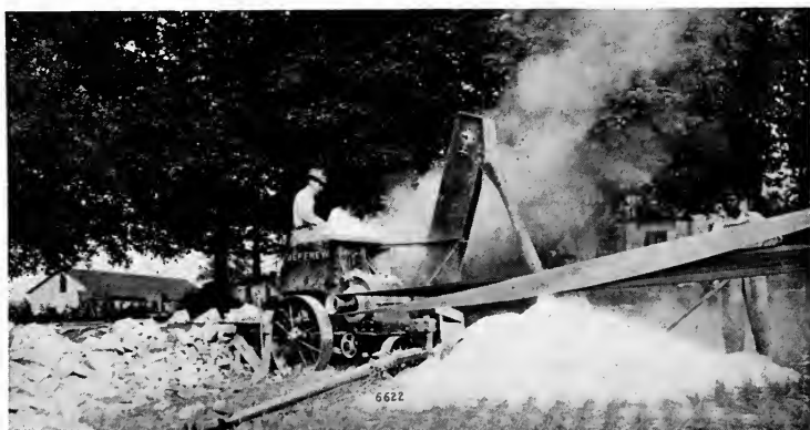
Fig. 21. A Portable Lime Grinder in Action.
