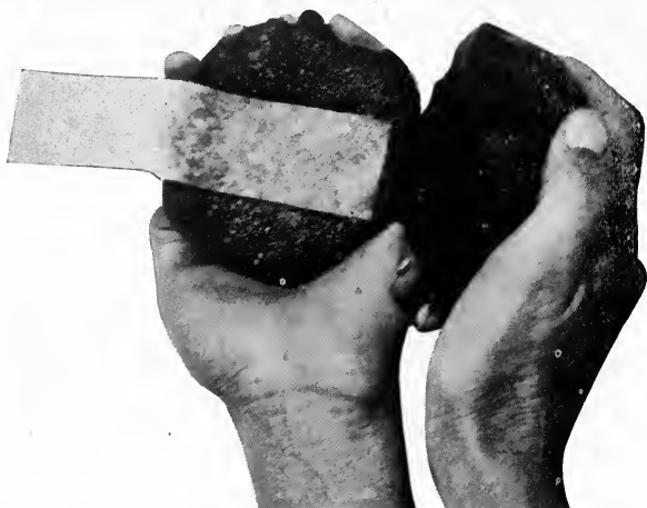
Fig. 19. The blue litmus paper turns pink when placed in contact with acid soil.
