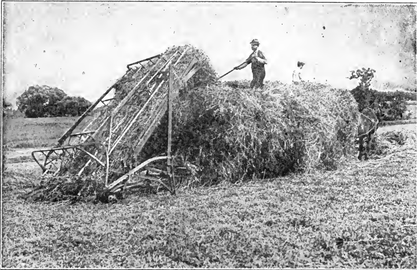
FIG. 85. Those who favor the hay loader usually store their hay in shed or barn. It gathers hay from the windrow or the swath.—[Courtesy Emerson-Brantingham Implement Company.]
