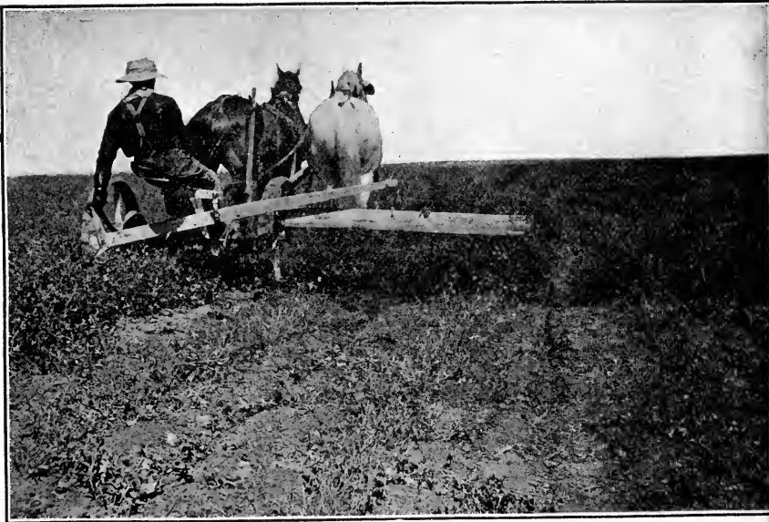
FIG. 214. A mowing machine with dropper attachment in operation in a field of rowed alfalfa. Extension guards, that extend out farther than the regular guards and pick up the lower parts of the alfalfa plants, are useful in harvesting alfalfa in rows.—[Courtesy U. S. Department of Agriculture.]
