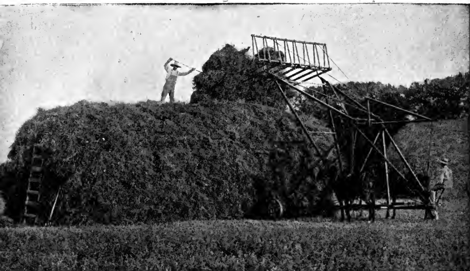
FIG. 67. The combination sweep rake and stacker will place hay on the stack in any spot desired. [Courtesy F. Wyatt Mfg. Co.]
