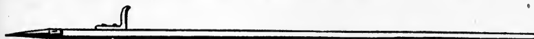
FIG. 307. A prod for locating runways of the pocket gopher and making openings for the introduction of poisoned bait.—[Courtesy Kansas Experiment Station.]
