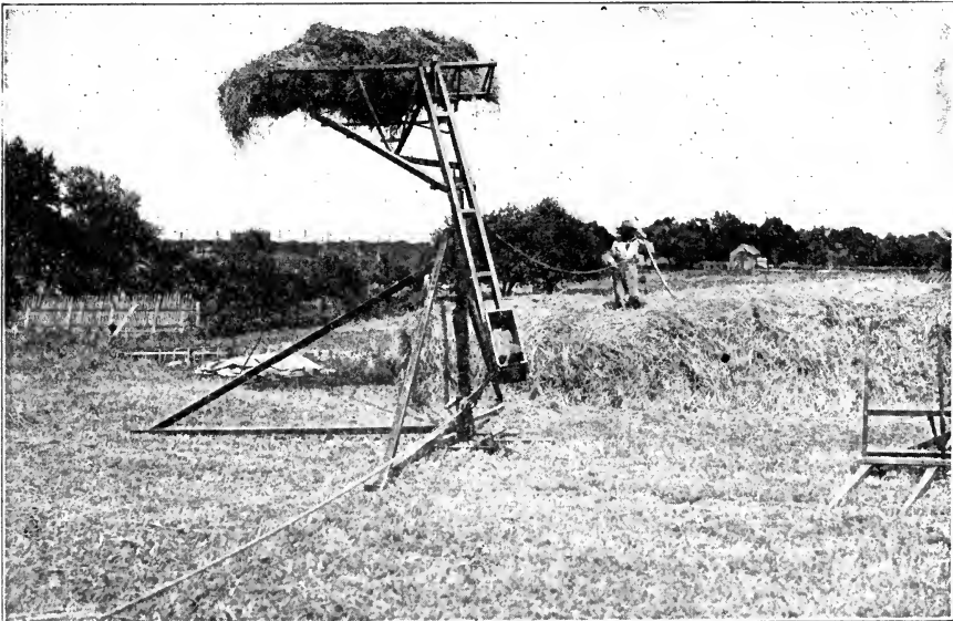
FIG. 69. The swinging stacker elevates and swings the load sidewise to the stack. [Courtesy Emerson-Brantingham Implement Company.]
