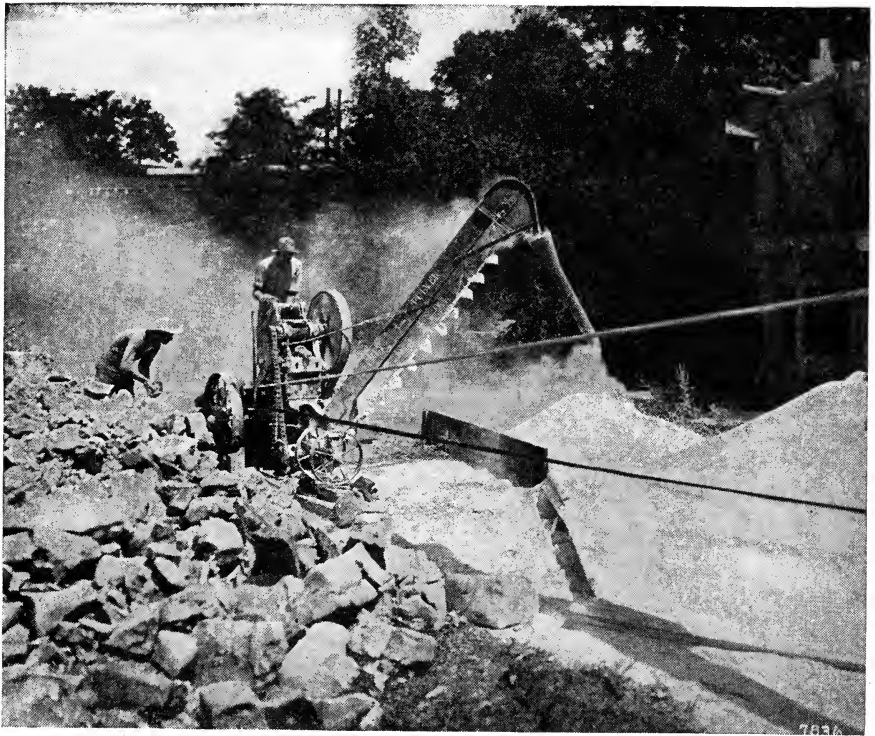
FIG. 19. There are few Kansas regions in which limestone may not be had within hauling distance, and farmers will do well to look into the cooperative purchase of portable lime pulverizers.—[Courtesy Power Farming .]
