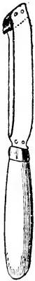
FIG. 38. Girdling knife, made of two thin steel blades with cleaner at a.
