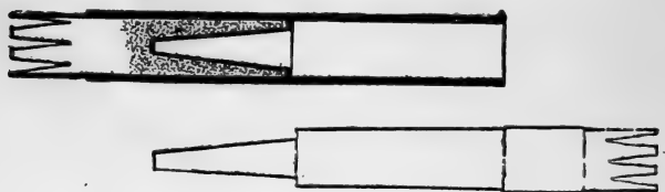
Fig. 15.—Sectional View of Doweled Ferrule.
