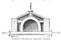
Fig. 2.—Sectional View showing the course of the circulation.
