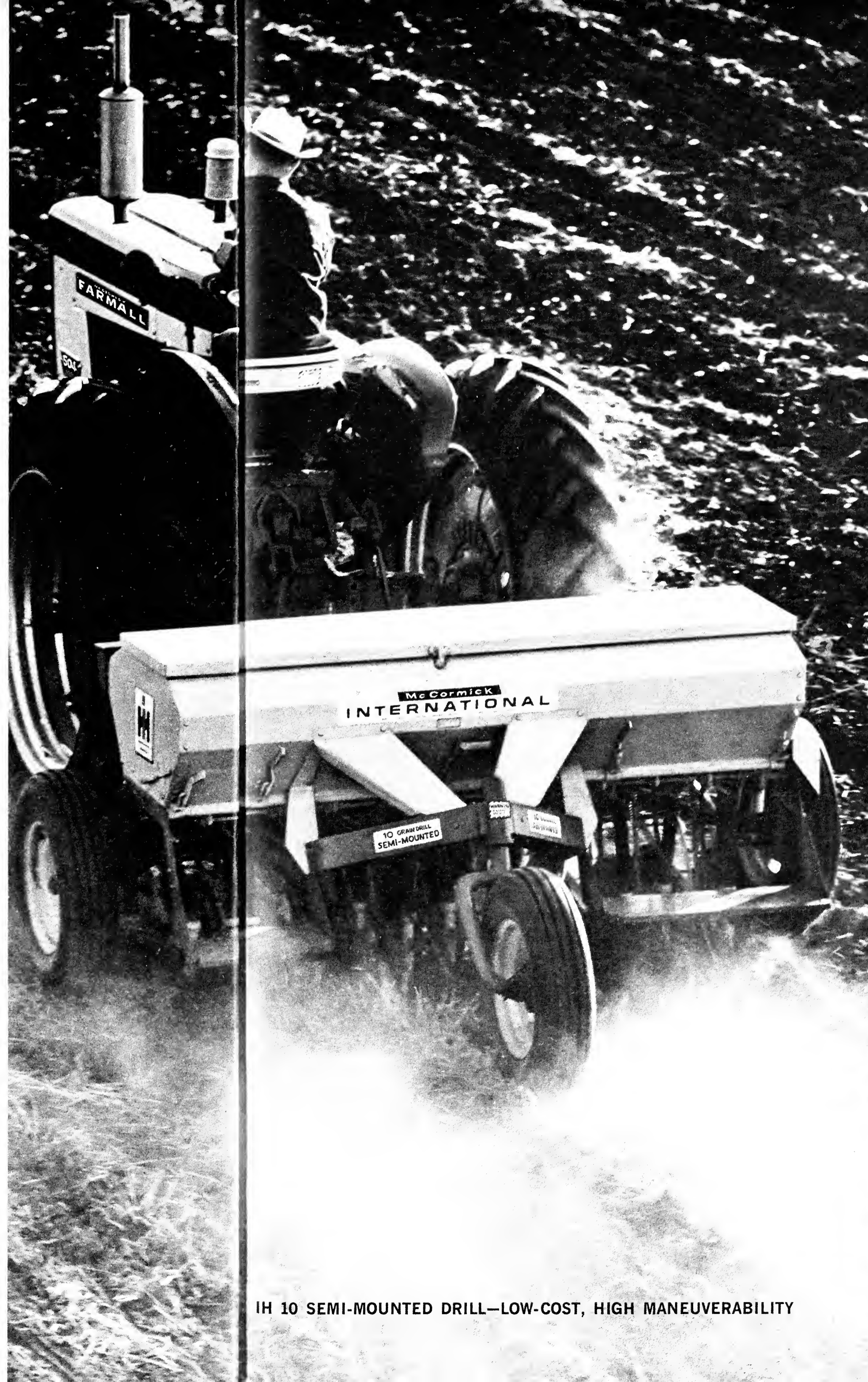
Precision feed cups and fluted rolls dole out seeds with one-at-a-time accuracy. Metering of seed is uniform across the width of the drill. Handy seed adjustment.
