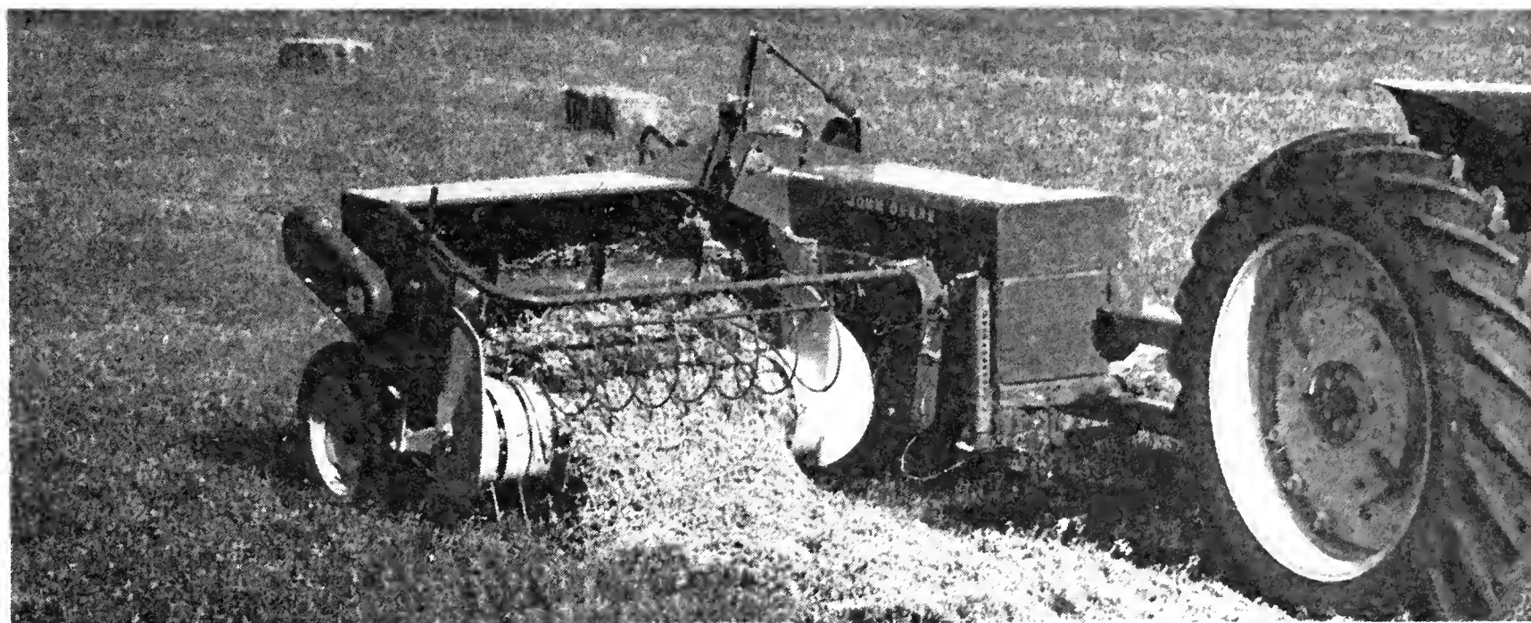
New 224 Series Balers have a pickup cylinder with five bars for faster feeding, faster travel speeds.
