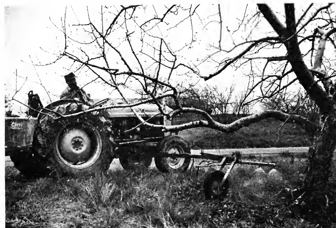
Otho Lewis built this rig that has "snap back" section of boom that prevents hurting tree trunk.
