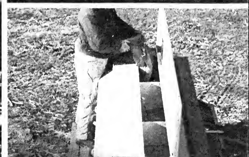
Super-big IH combination hopper holds a whopping 85 pounds of fertilizer and 1 1/4 bushels of seed per foot. Apply fertilizer at rates from 78 to 800 pounds per acre.
