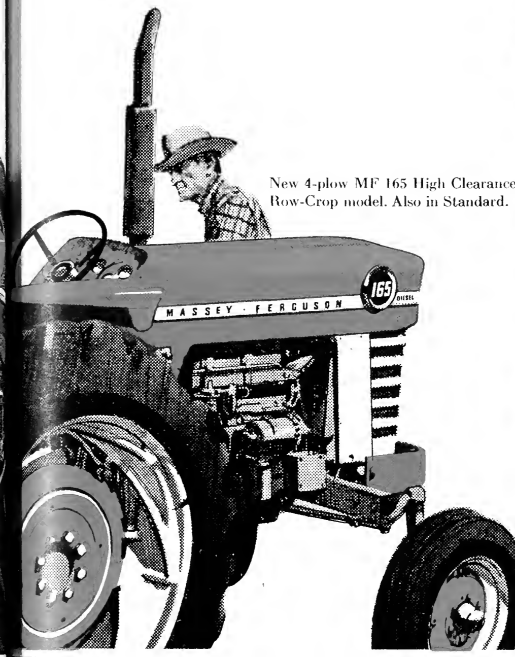
Advanced Ferguson System adds new work power to mounted and semi-mounted implements. Now with stepped-up hydraulics for more "muscle" and lift—more precise implement control—fast, automatic draft response to changing soil conditions.
