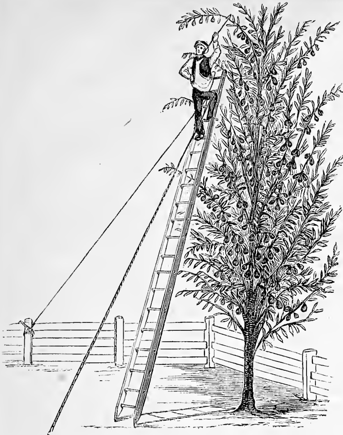
Fig. 1.—METHOD OF STAYING A LADDER.
