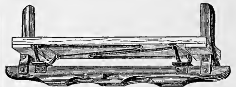
Fig. 2.—TORSION WAGON-BOX SPRING.
