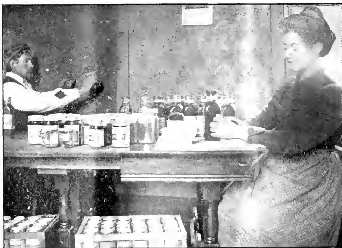
FIG. 3.—LABELING AND TIN-FOLIING WITH A CAPPING STRAP (TIN-FOLIING SHOWN AT LEFT)
