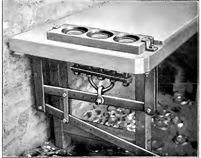
Fig. 5—Packing Ring Mold with Arbors Withdrawn.
