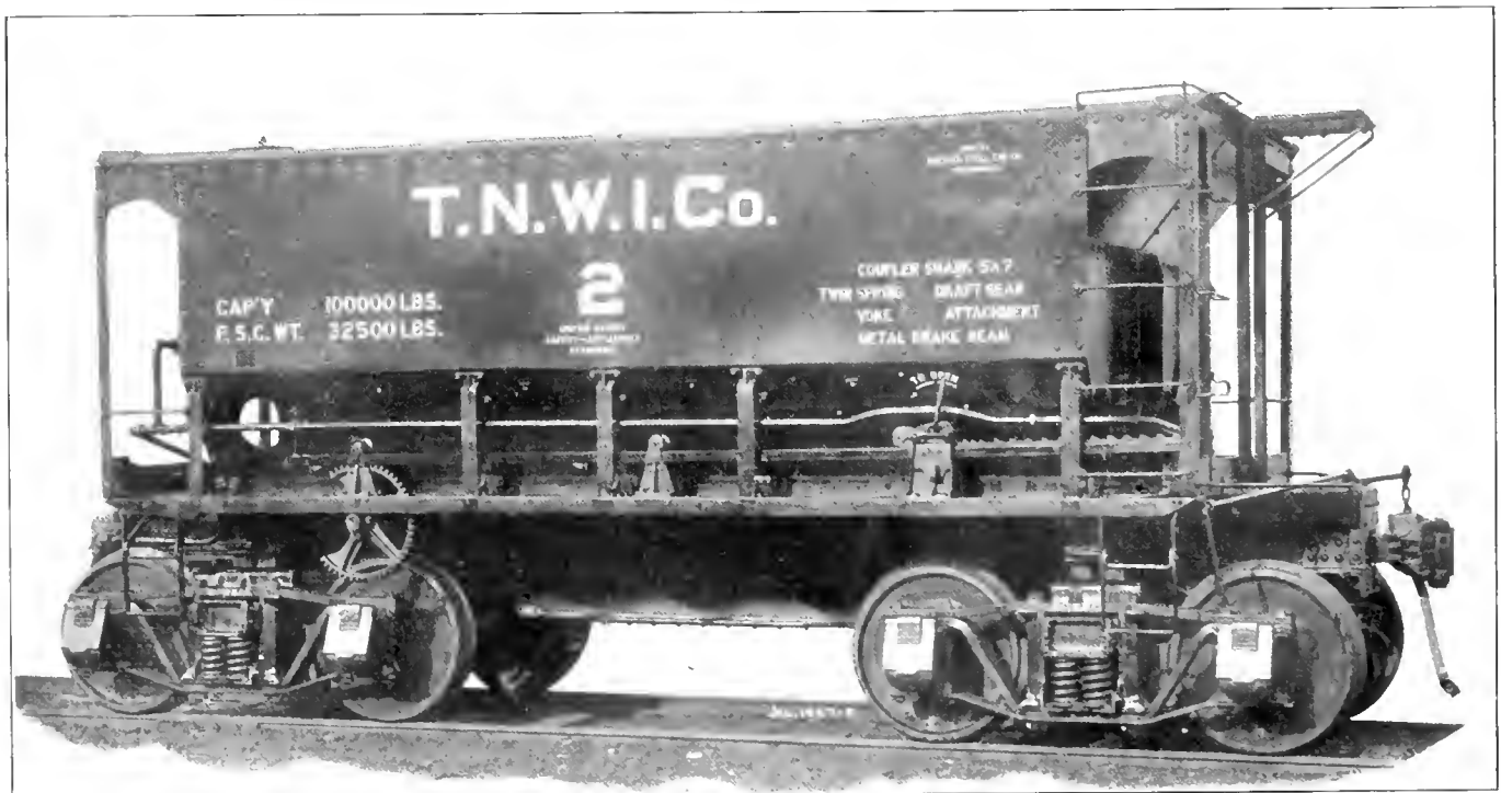
Steel Self-Clearing, Quick-Dumping Ore Car for the Northwest.
