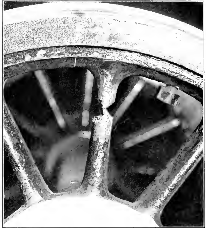
Fig. 14—Cracked Wheel Spoke Chipped Preparatory to Welding.
