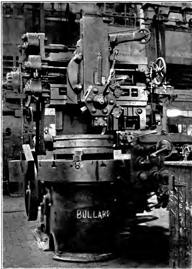
Finishing a Piston Head at the Macon Shops.
