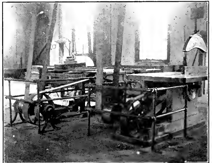
Fig. 7—Railing and Guards for Safeguarding Woodworking Machines.
