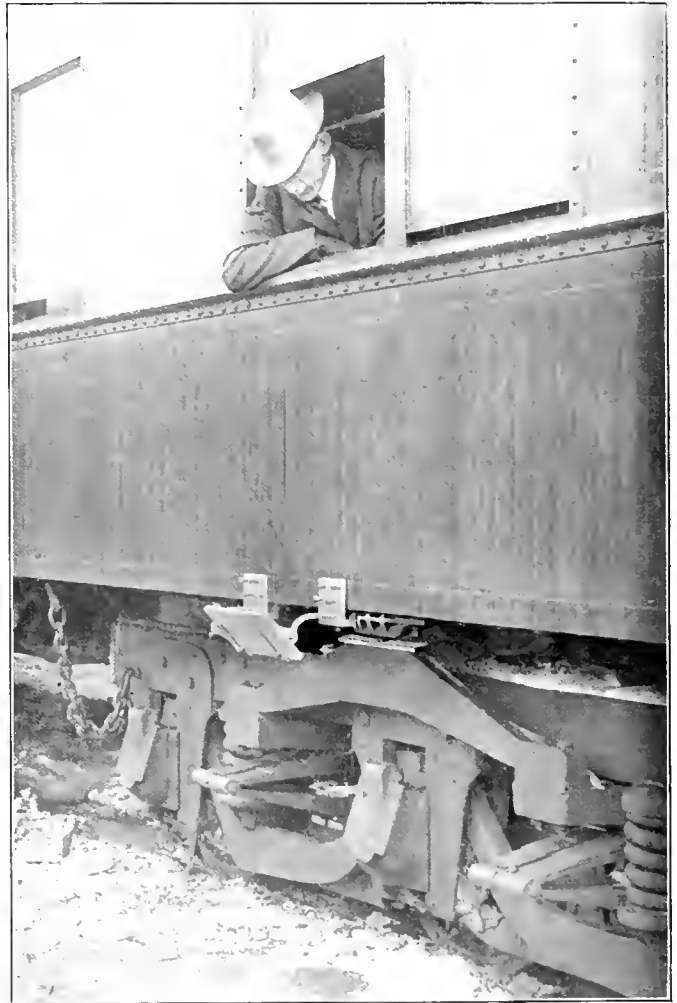
Mirror for Inspecting Side Bearing Motion.
