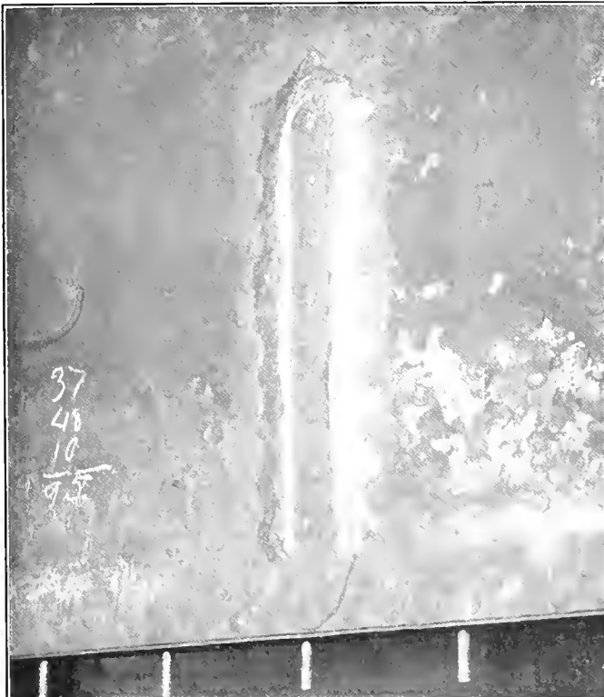
Fig. 10—Side Sheet Patch Welded to Firebox.
