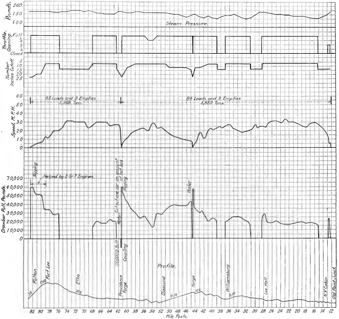
Graphical Record of a Recent Test of a Chesapeake & Ohio Mikado Locomotive.
