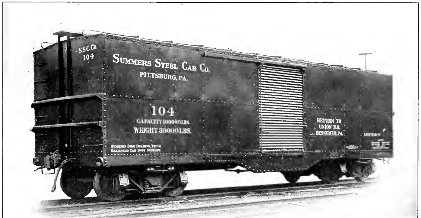
All-Steel Box Car Similar to Those Ordered by the Bessemer & Lake Erie, Although Not Quite as Long.
