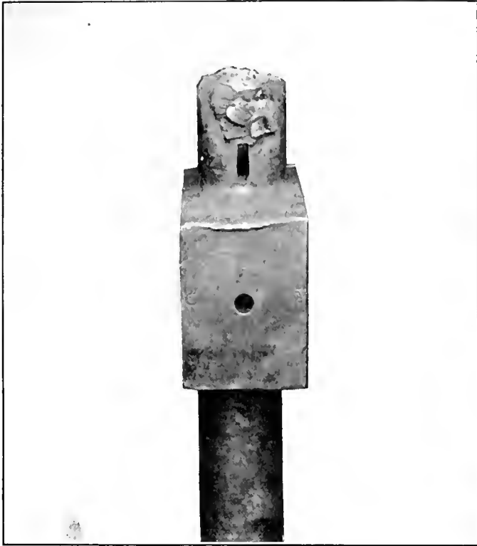
Fig. 12—Valve Rod Guide After Welding.
