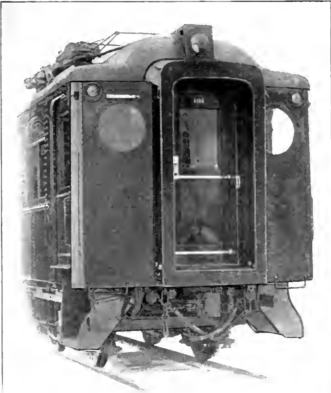
Vestibule of All-Steel Suburban Car.
