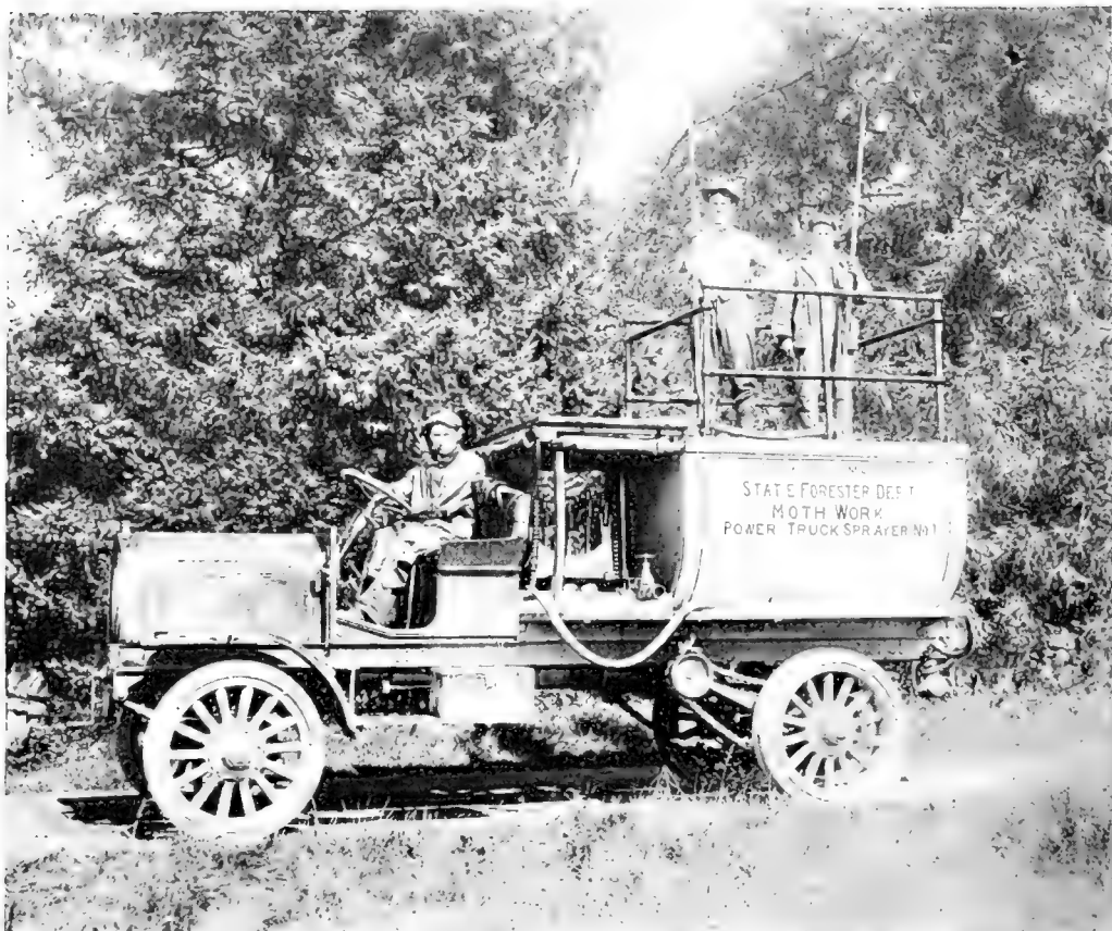
A CLOSE VIEW OF THE NEWLY INVENTED POWER-TRUCK SPRAYER. SAME POWER AS THE ABOVE, BUT DOES AWAY WITH HORSES AND DRIVER, AND THE ENGINEER BECOMES THE CHAUFFEUR. TANK AND PUMP ARE EASILY REMOVED AND THE TRUCK THEN IS USED THE SAME AS ANY TRUCK.
