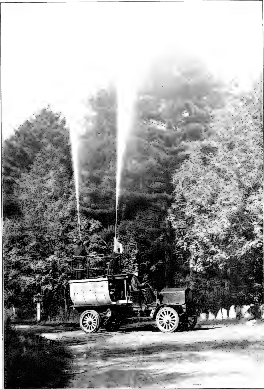
THE FIRST POWER-TRUCK SPRAYER EVER INVENTED. BUILT BY THE MASSACHUSETTS STATE FORESTER IN 1911 FOR SPRAYING IN THE GYPSY AND BROWN-TAIL MOTH WORK. THE WHOLE OUTFIT WAS DESIGNED AND BUILT FOR THIS WORK, AND PROMISES TO REVOLUTIONIZE THE QUESTION OF SPRAYING, PARTICULARLY ROADSIDE, PARK AND SHADE TREE WORK, IN COMBATING INSECT AND FUNGUS DEPREDATIONS. IT CAN BE USED FOR FOREST FIRE WORK AS WELL. THE SAME ENGINE THAT PROPELS THE TRUCK ALSO IMPARTS THE POWER FOR SPRAYING.
