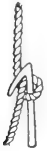
FIG. 39.—Proper way to make first "hitch" of rope on hook of counterweight.
