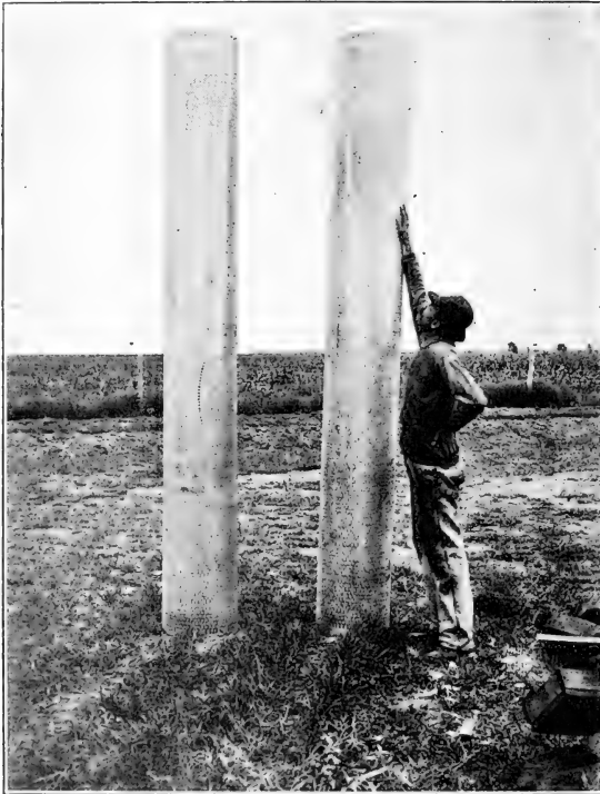
Fig. 1—Well strainers made of slotted galvanized iron. These strainers are 15 inches in diameter, and ten feet long, provided with 3-16 by 1 1-4 inch hit and miss slots, punched before the steel is galvanized. The strainers shown in the diagram were made of No. 18 gage sheet steel.
