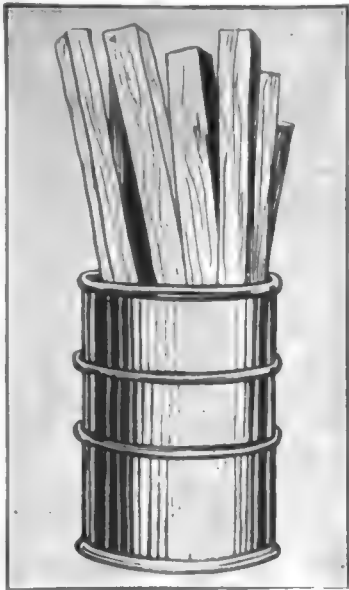
Showing tank treatment of timber with Grade-One Creosote Oil
