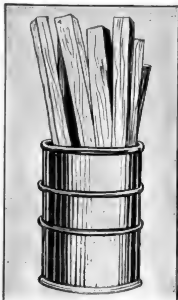
Showing tank and treatment of timber with Grade-One Creosote Oil
