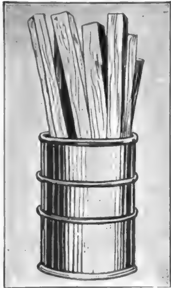
Showing tank treatment of timber with Grade-One Creosote Oil
