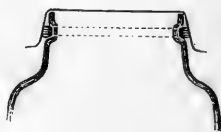
Fig. 165.—Section of top of Jar, with India-rubber band; place of India-rubber shown by dotted line.
