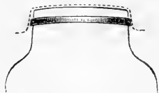
Fig. 164.—Top of Jar, with India-rubber band; place of tin cap shown by dotted line.
