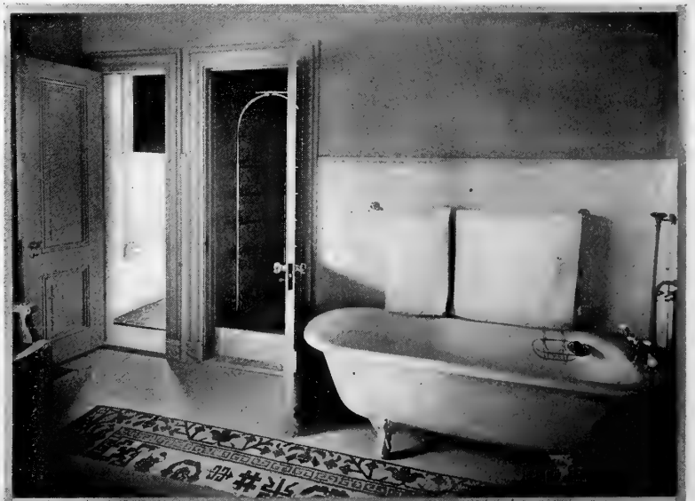
A closet shower opening out of the bathroom
