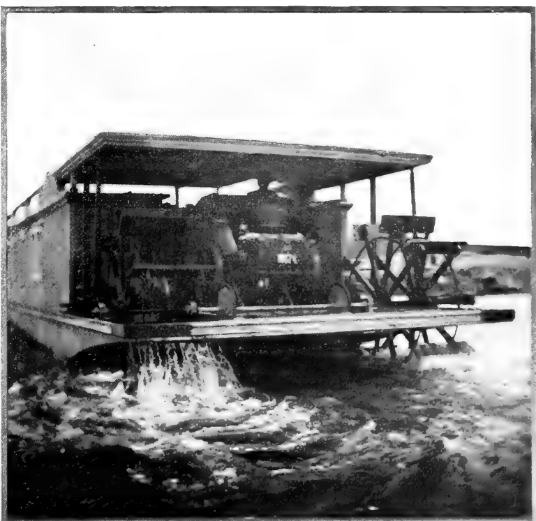
This shows the spurred sprocket wheels on the paddle-wheel axes
