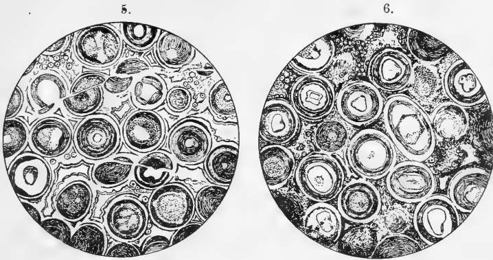
FIGS. 5 and 6.—Micro-sections of Siliceous Oolite from Pennsylvania, magnified 10 diameters.
