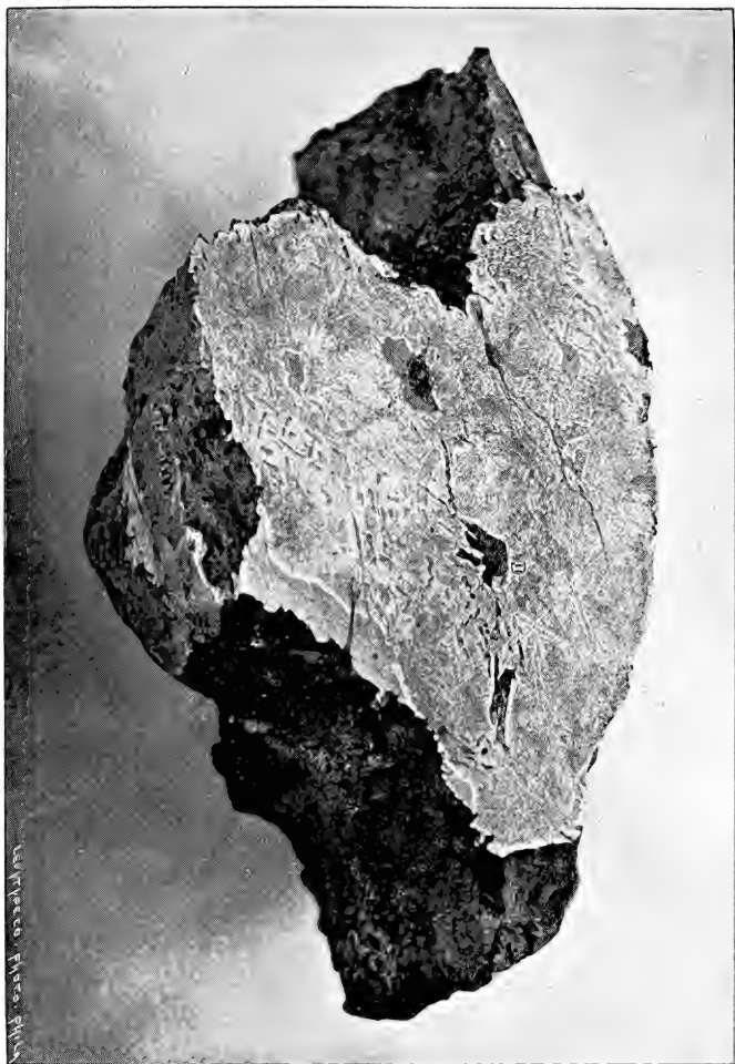
Polished Surface of Meteoric Iron from Cañon Diablo, Arizona, showing Widmanstätten figures. A small black diamond is shown protruding near one side of the central black cavity; at D, a circle of scratches made by small loosened diamonds can be seen near this spot.
